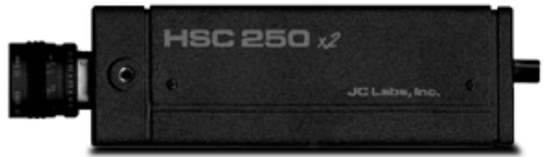
The CCD image pick-up on the HSC-250 x2 features 765 pixels across by 246 pixels, giving a resolution of 570 television lines horizontally in an RS-170 compatible format. The full resolution of the camera is available at any speed from 60 to 250 pictures per second.
